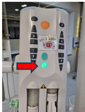
(B) Manually check for air in front of the auto injector and press the air check button.
