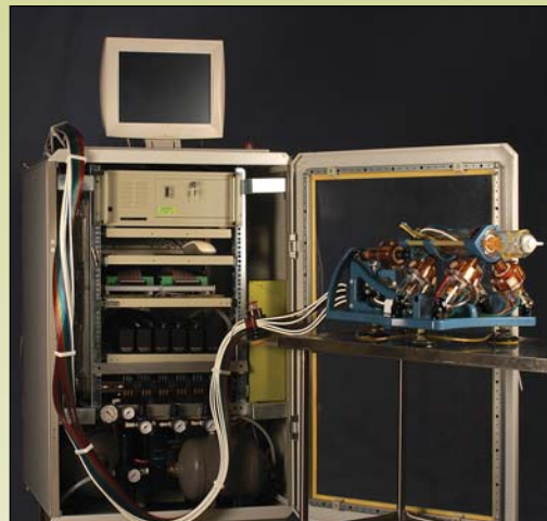
MrBot is a plastic, electricity-free robot. The robot is connected, with air hoses and optic fibers, to a control cabinet located outside the MR imaging room. The cabinet contains all control electronics and communicates with the robot through electro-optical and electropneumatic interfaces.
