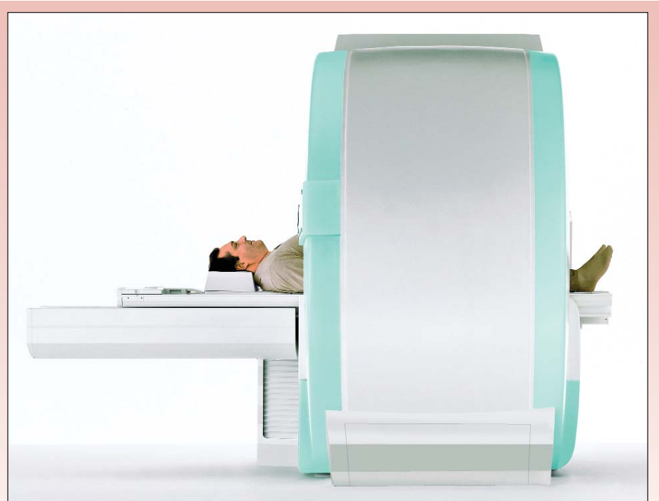
The MAGNETOM Espree is the first 1.5 Tesla MR imaging unit offering “scan equity” for obese patients. It is the first 70 cm bore in MR and has a 550-pound weight limit. Espree offers at least 10 cm more vertical space than low-field, vertical-field open MR systems.
