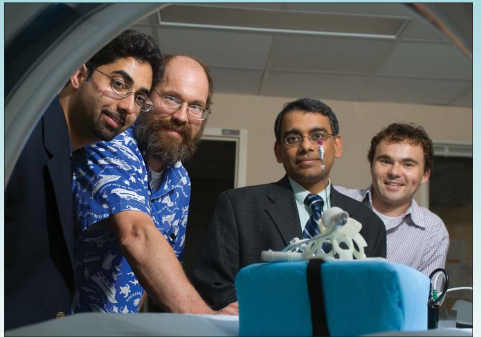
Inventors of Robopsy (left to right) Nevan Hanumara, Alexander Slocum, Ph.D., Rajiv Gupta, M.D., and Conor Walsh, pictured with the robotic system (forefront) that aids in CT-guided percutaneous procedures. Designed to sit over a patient's chest during a CT scan, the device grips, orients and inserts a biopsy needle or ablation probe while that patient remains inside the CT gantry.
